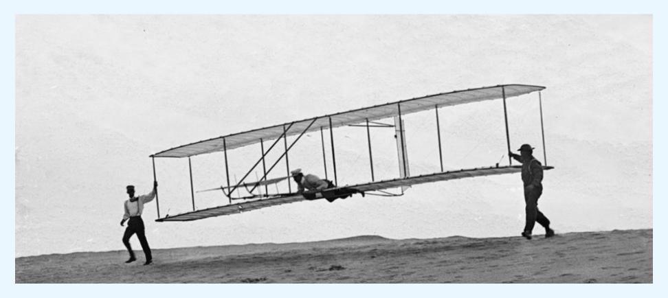
After initial knowledge building using kites, they initiated a logical series of experiments with gliders that developed design innovations to achieve sustained lift and control sufficient for successful powered flight
